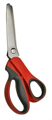
Pinking Shears feature notched, sawtooth blades that leave a zig-zag pattern along your fabric edge. This limits the length of frayed threads to help prevent unraveling. These 9 1/2" Pinking Shears have stainless steel blades and an ergonomic handle. They can also be used with ribbon, paper and other materials to add decorative edging.
