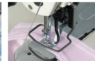
M type (Bartacking shoulder of running shirt)
