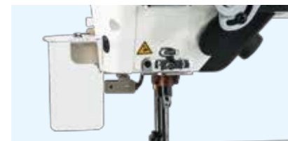
① Eye guard with an open/close sensor
